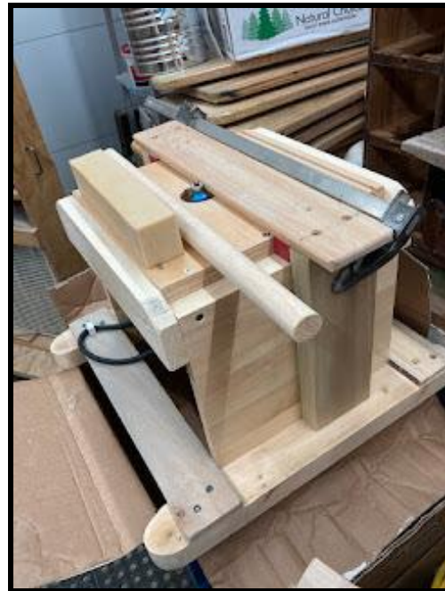
A simple set up for any router table to round over the ends of dowels.
